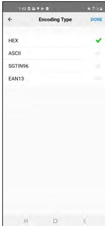
Sets the encoding type of the inventory results. The page displays inventory results in this encoding type.
