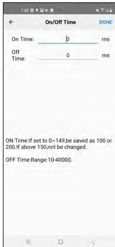
RFID power On Time (transmission time) / Off Time (idle time) can be set.
